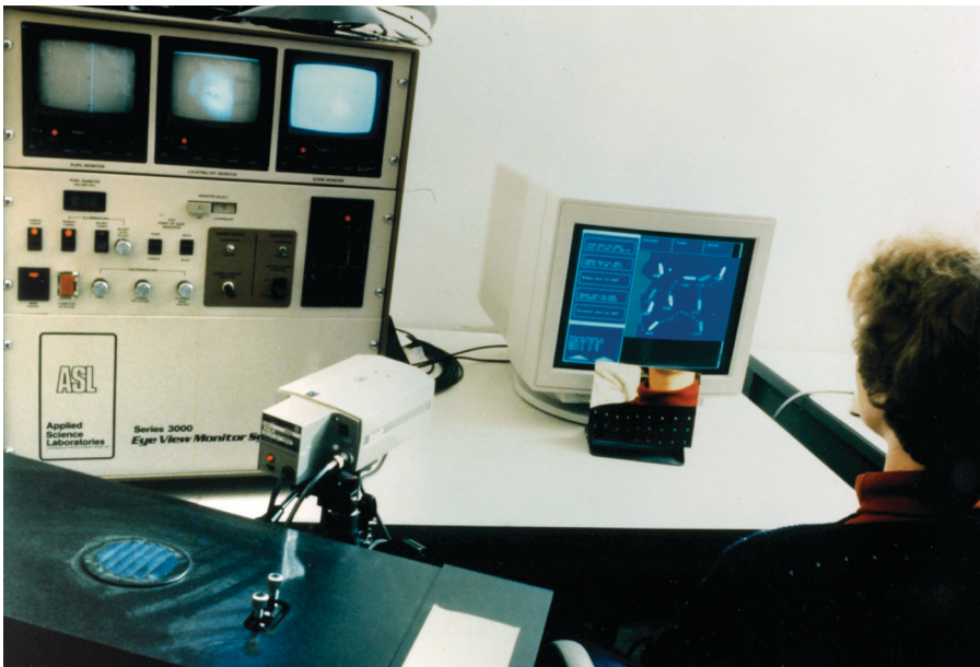
Figure 1. State-of-the-art eye-tracking equipment in the 1980s: the Eye View Monitor from Applied Science Laboratories (ASL).
